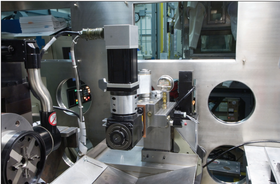
Milling tool attachment mounted in the tool post inside the glovebox.
