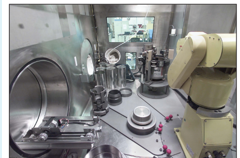
The hot-side chamber of the robotic integrated packaging system (RIPS) glovebox. RIPS is also known as the robotic packaging (ICAN) module.
