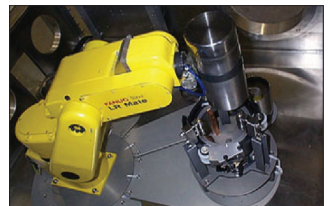
Automated packaging of special nuclear material allows for significant reductions in worker dose and greater safety.
